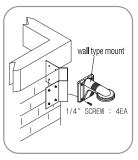
3. Fix the wall type mount(STB-270PWV) with four 1/4 inch screws.
